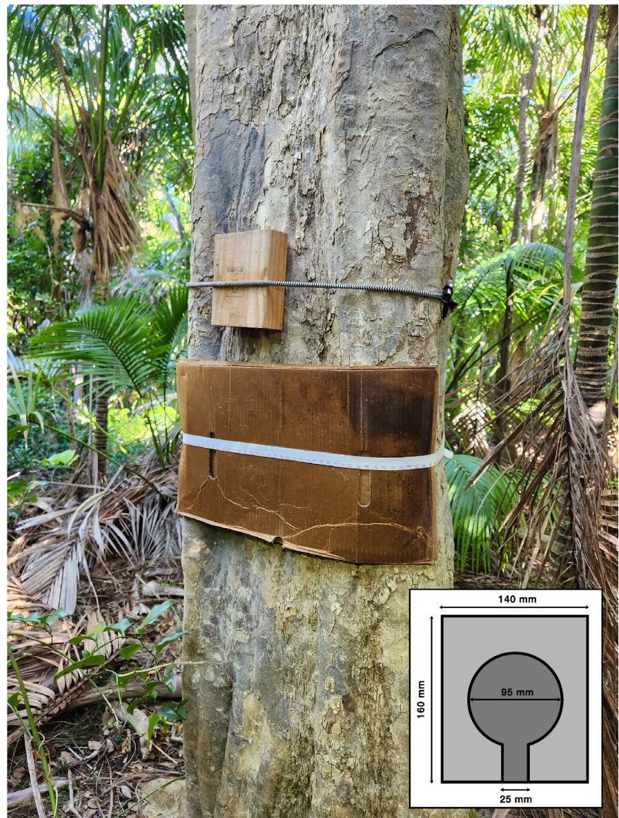
Fig. 2 Cardboard tree wrap and wooden tree block strapped to a tree to mimic exfoliating bark and a tree hollow, respectively. Inset: schematic representation of a tree block. Dark shaded region incised to a uniform depth of either 9 mm or 17 mm. When deployed, the incised surface was positioned facing inwards against the tree with the opening directed downwards
